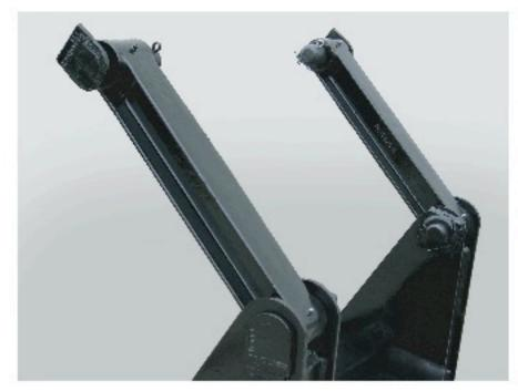
Shown is the heavy duty cast lift arms. These arms easily attach directly to the body using 4140 grade, 1 1/2" hinge pins. The arms have easily accessible zerk grease fittings.
